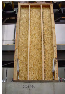
Figure 6.2-1 Egmented shear wall with studs, sheathing, and posts and tie-down connectors at each end.
