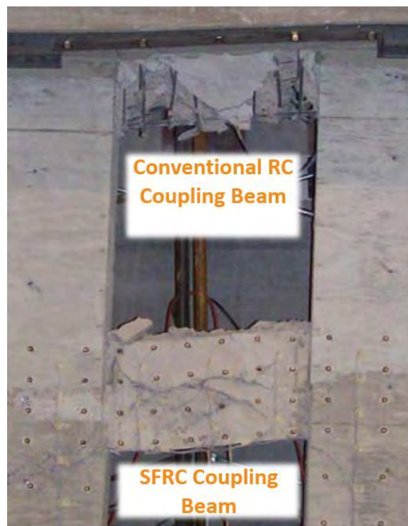
Figure 2.1-16 Comparative Testing [Figure Credit: Lequesne, 2011]
