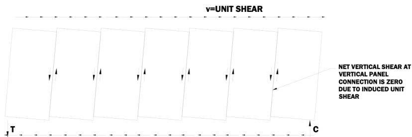
Figure 6-1. Illustration of Rocking Behavior of Seven Individual Panels in A Multi-panel CLT Shear Wall Designed in Accordance with SDPWS-21 Appendix B
