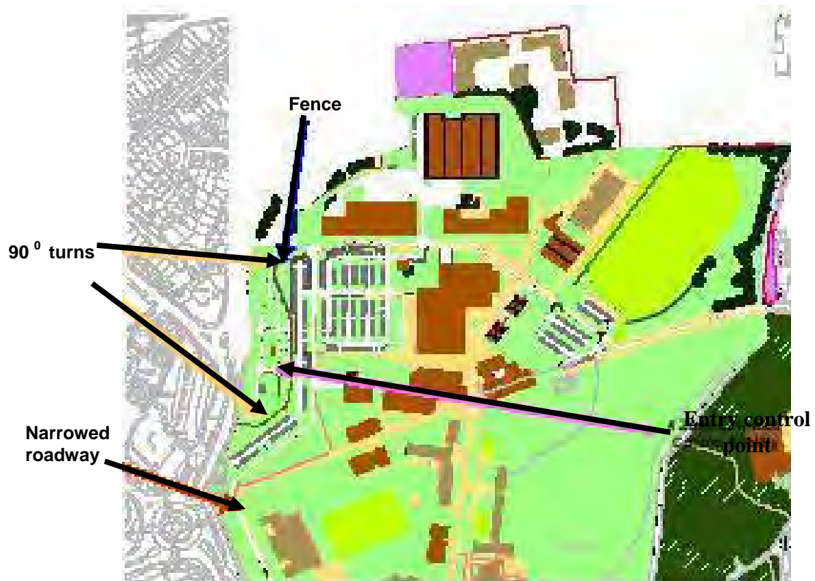
Figure 5-3. Road Modifications to Reduce Speed
