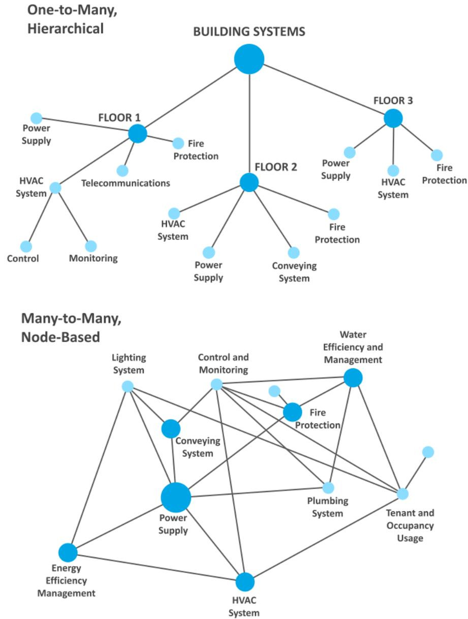
Figure 9 – Comparison between BIM (Above) and Digital Twin (Below) Native Data Structures
