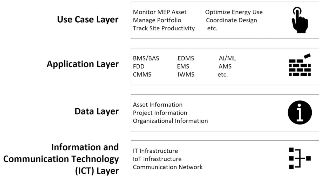
Figure 10 – Data framework to decouple data from applications
