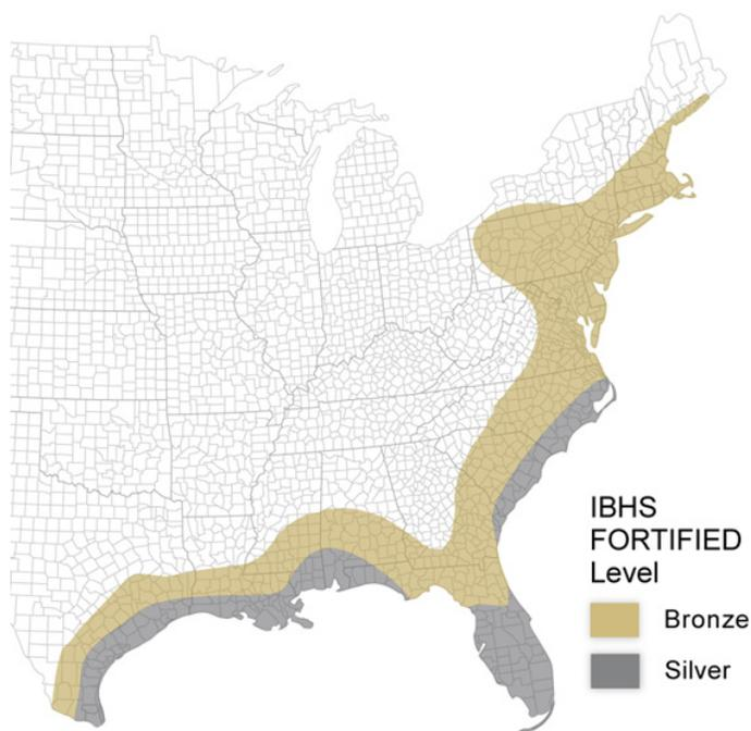
**FIGURE 2.** Maximum level of the IBHS FORTIFIED Home Hurricane design for new construction where the incremental benefit remains cost-effective.
